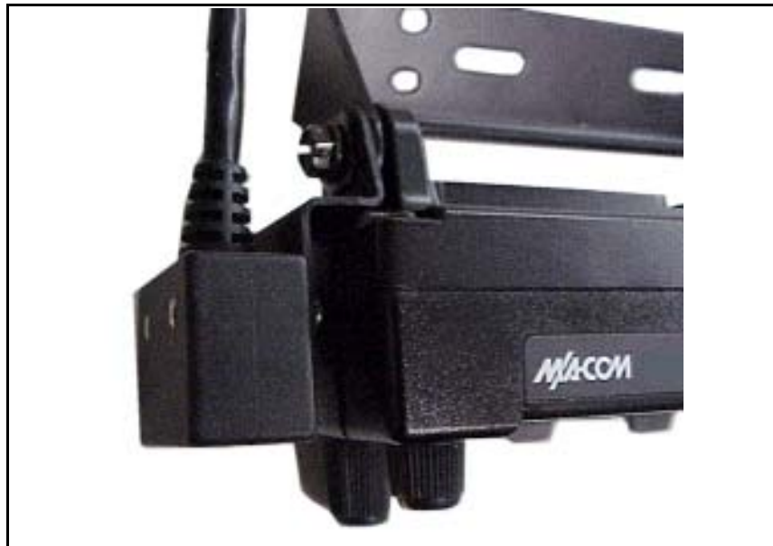
Figure 9-10: Pigtail Bracket Installed on Control Unit
