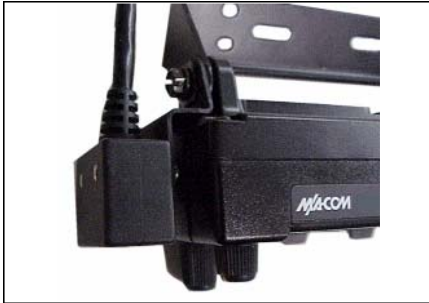
Figure 9-10: Pigtail Bracket Installed on Control Unit
