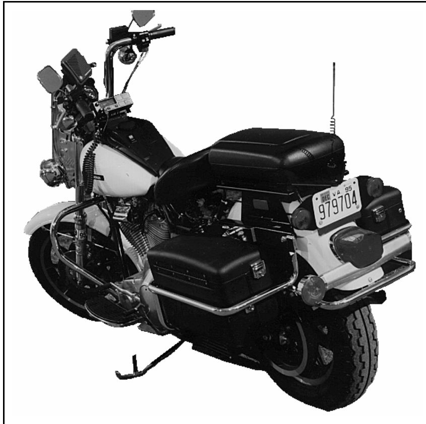
Figure 3-1: Typical M710 IP Motorcycle Installation
