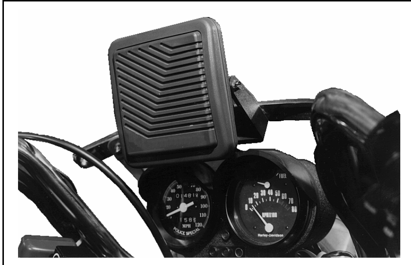
Figure 7-3: Typical Speaker Mounting
