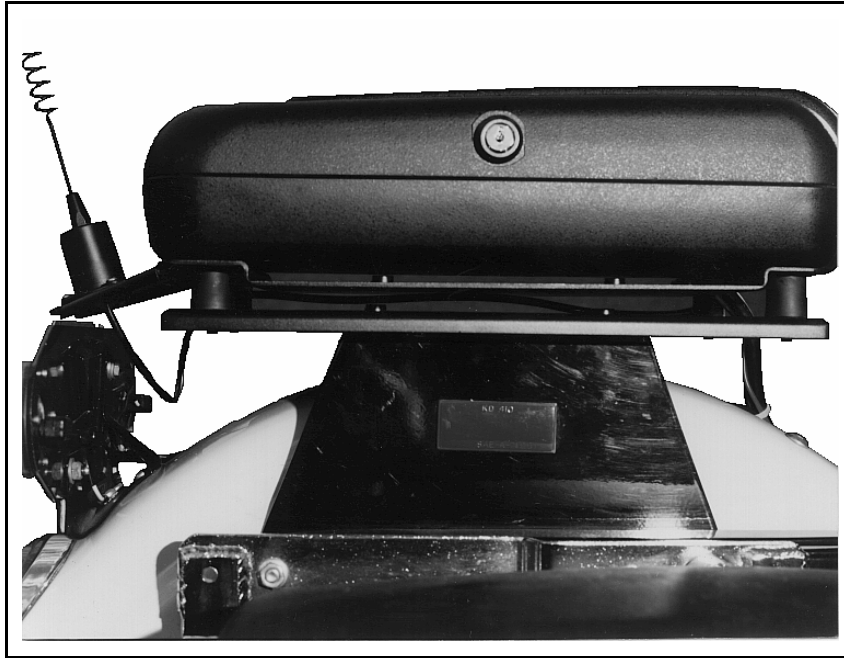
Figure 6-3: Case Mounting Bracket and Case Assembly
