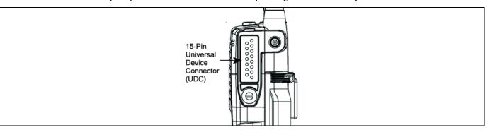
Figure 7-7: XG-75 15-Pin Universal Device Connector
