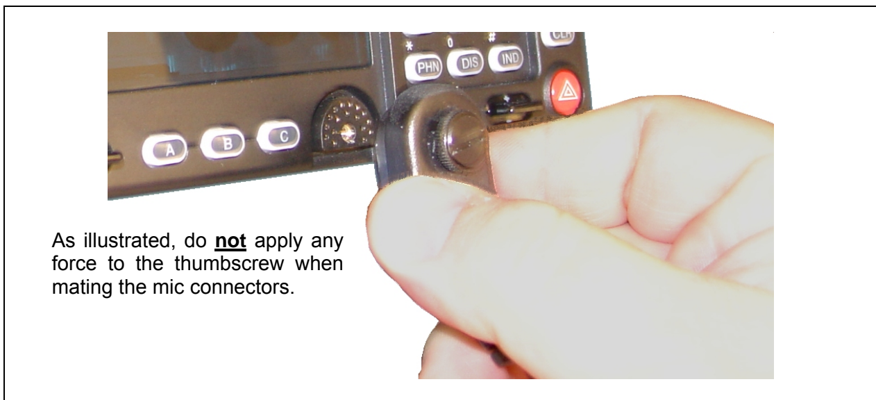
Figure 10-1: Attaching the Microphone to the CH-721 Control Head
