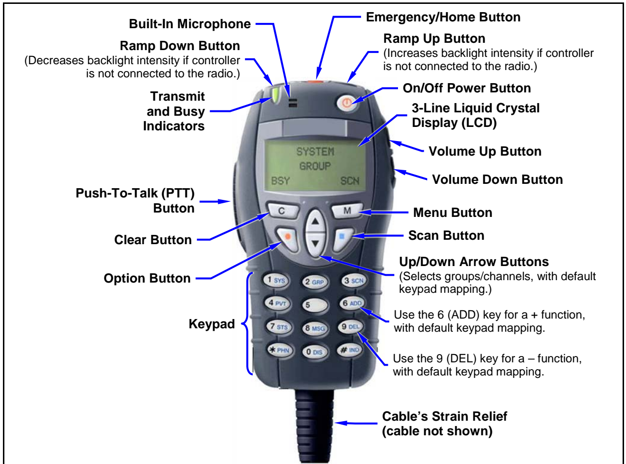
Figure 8-14: HHC-731 Hand-Held Controller Front View
