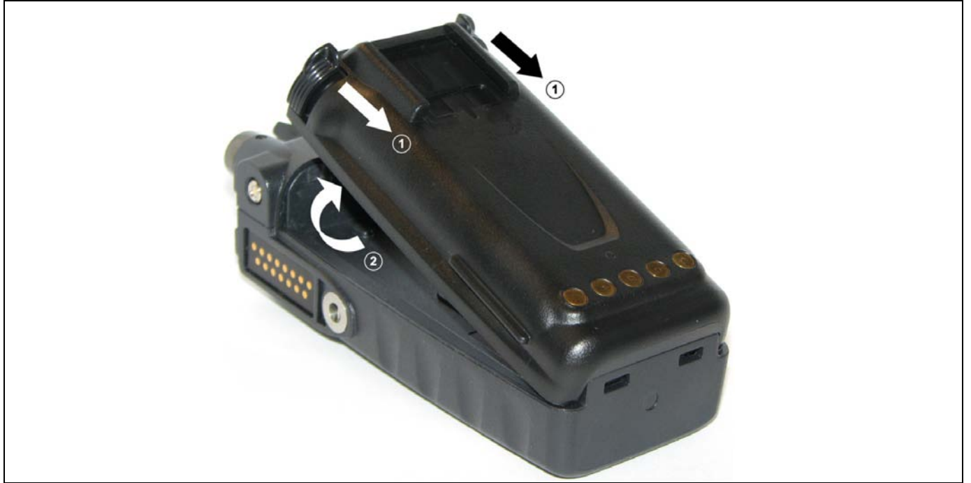
Figure 4-1: Removing the Battery Pack
