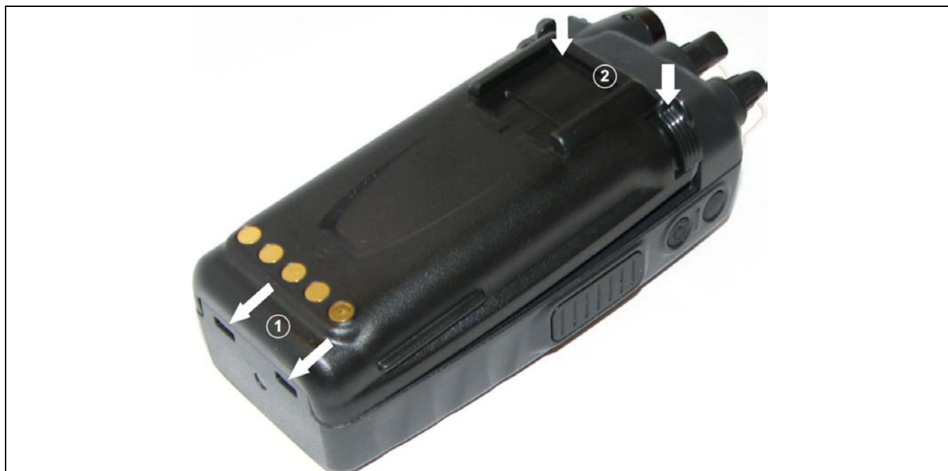
Figure 4-2: Attaching the Battery Pack
