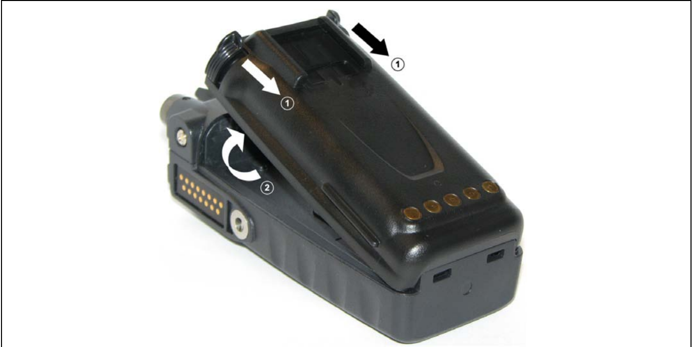
Figure 4-1: Removing the Battery Pack
