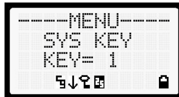
Figure 8-4: System Encryption Key Display
