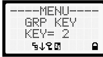
Figure 8-5: Group/Channel Encryption Key Display
