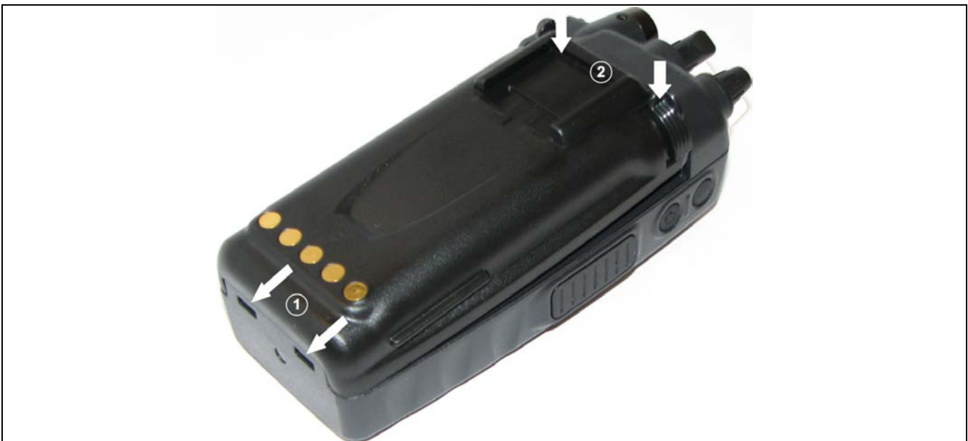
Figure 4-2: Attaching the Battery Pack
