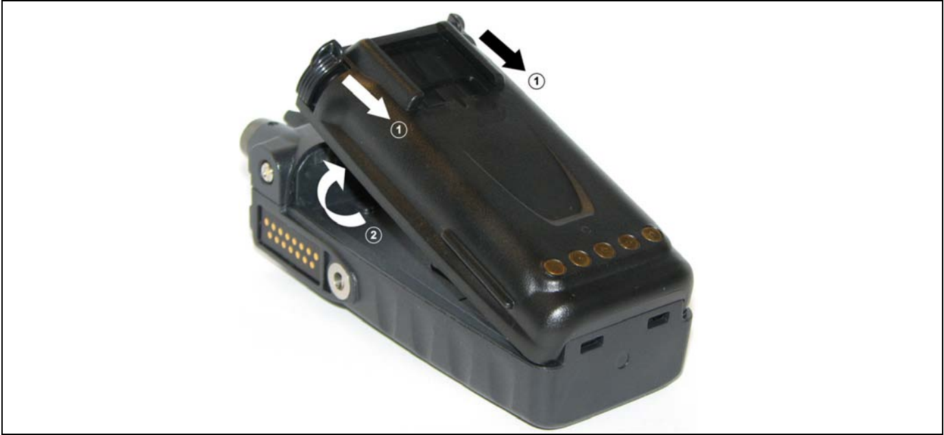
Figure 4-1: Removing the Battery Pack
