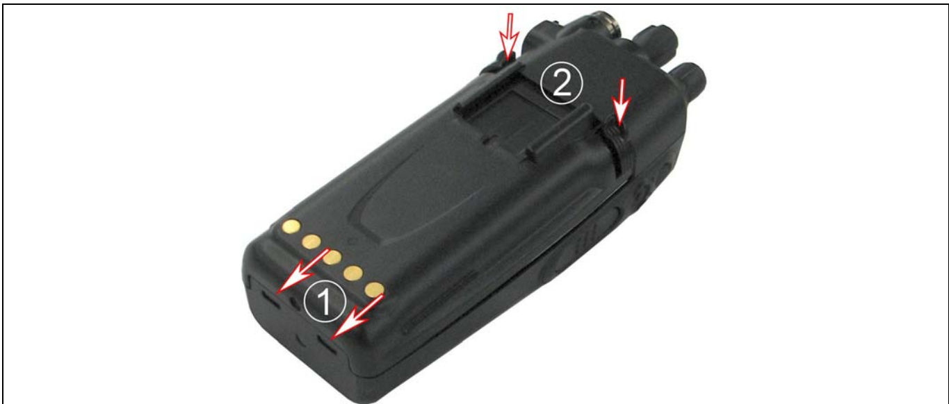
Figure 5-2: Attaching the Battery Pack
