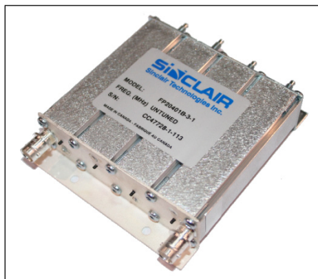
Figure 4-7: RF Front End Preselector
