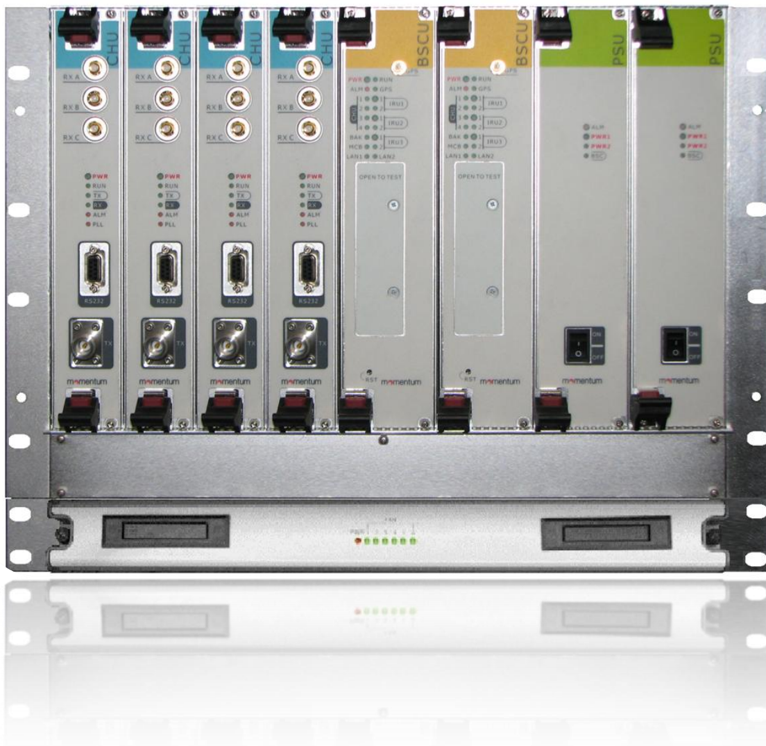
Figure 3-1: Transceiver Shelf and Fan Assembly (Configured with 4-RF Channels)
