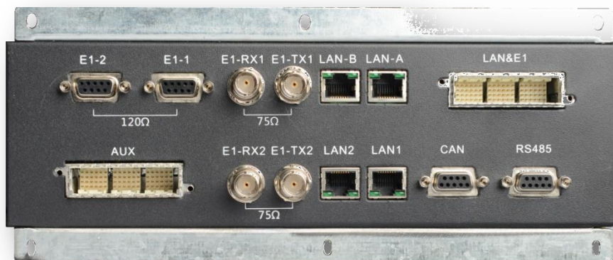
Figure 3-9: Extended Interface Board (Internal Connections View)
