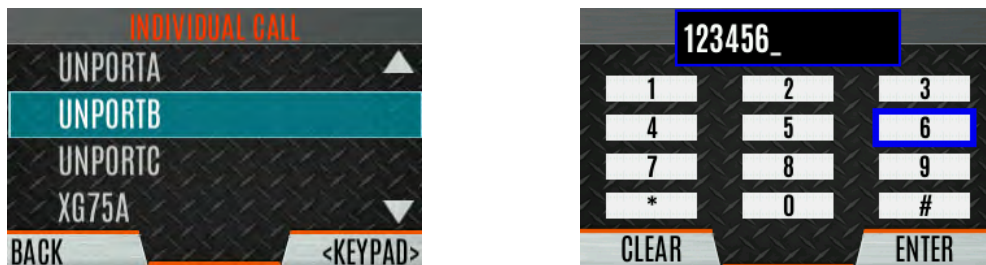
Figure 4-2: Using the Soft DTMF Keypad
