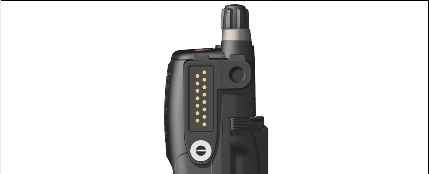
Figure 5-1: XG-25P 15-Pin Universal Device Connector
