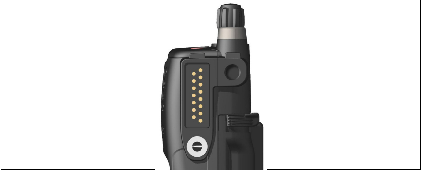
Figure 5-1: XG-25P 15-Pin Universal Device Connector
