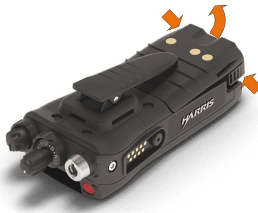
Figure 4-2: Remove the Battery
