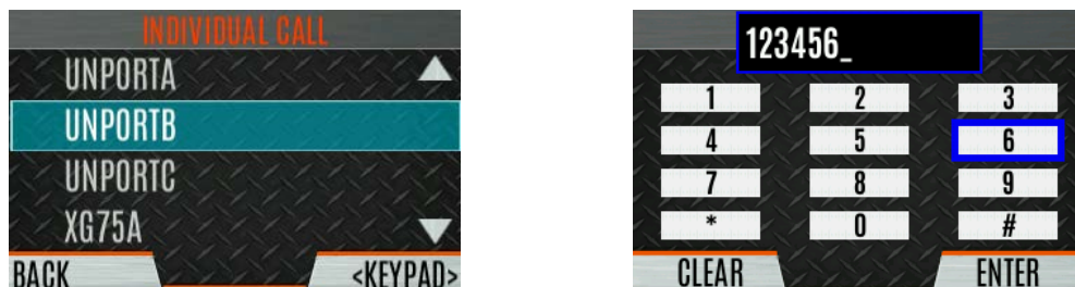
Figure 5-2: Using the Soft DTMF Keypad
