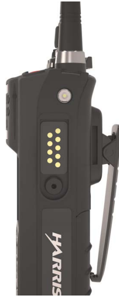
Figure 4-5: Universal Device Connector
