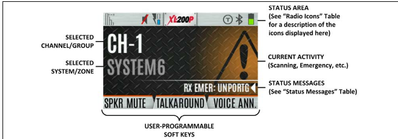
Figure 5-4: Sample Idle Front Display
