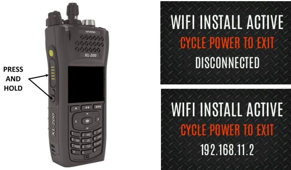
Figure A-5: Enable Wi-Fi Programming Mode on XL-200P
