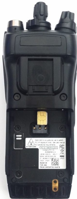
Figure 4-4: SIM Card Installation
