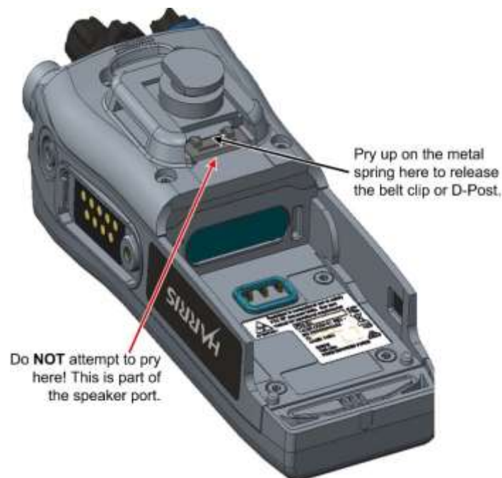
Figure 4-3: Remove Belt Clip
