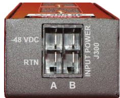
Figure 4-13: EA-555019-003 --48 VDC Low Power DC Distribution Strip
