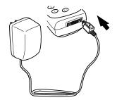
The terminal automatically starts charging the battery when you attach the charger. The following indicate charging:
