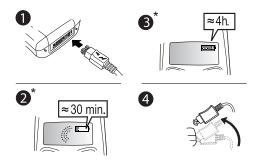
\* It may take up to 30 minutes for a new or fully discharged battery to indicate charging. It takes about 4 hours to fully charge a battery for the first time.
