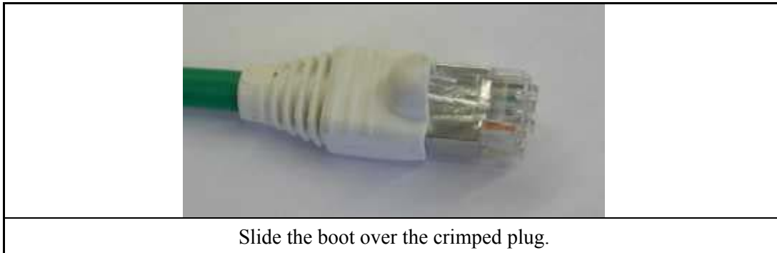
Figure D-18: Connector Termination, Slide on Boot Cover
