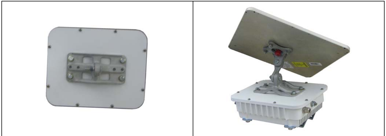
Figure 7-2: Mounting a Directional Antenna to the VIDA Broadband Client
