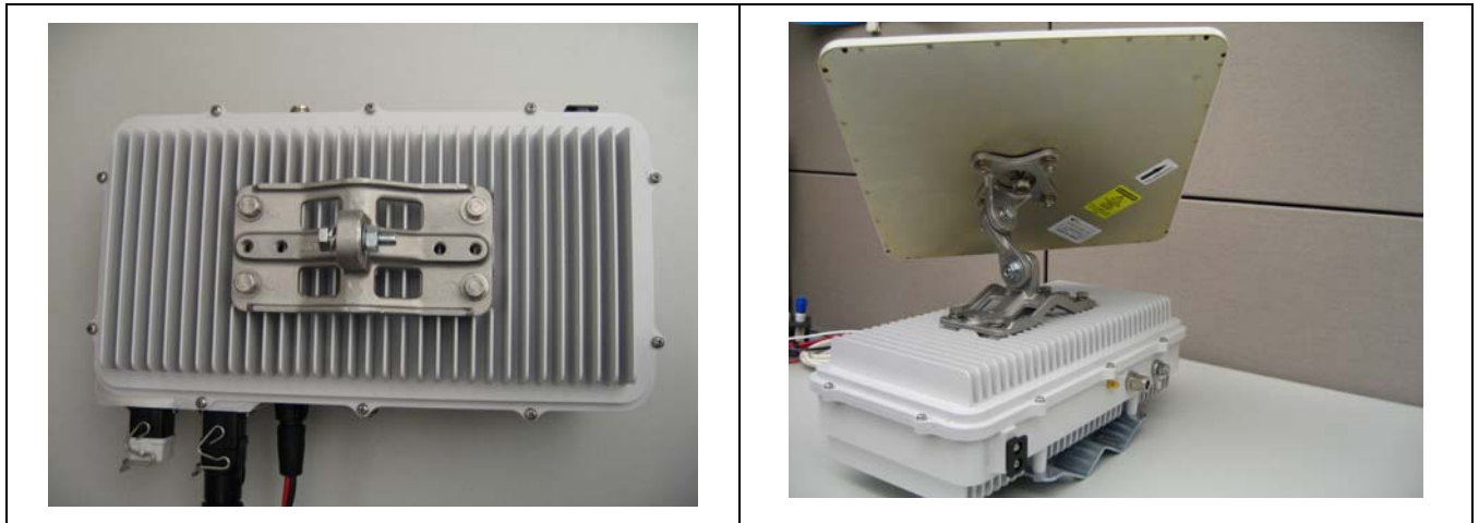
Figure 7-4: Mounting a Directional Antenna to the VIDA MAX Base Station
