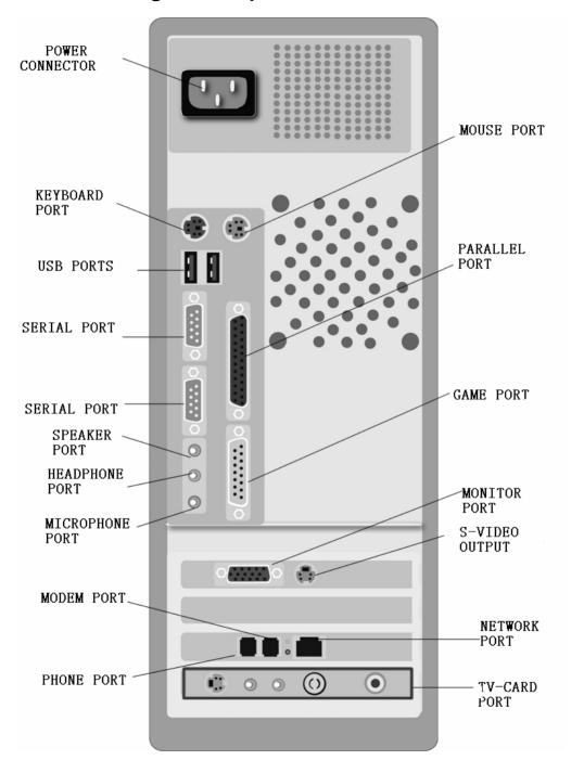
Follow the setup poster to set up your computer. The locations and the colors follow as PC99 model. Match the colors to connect the components.
