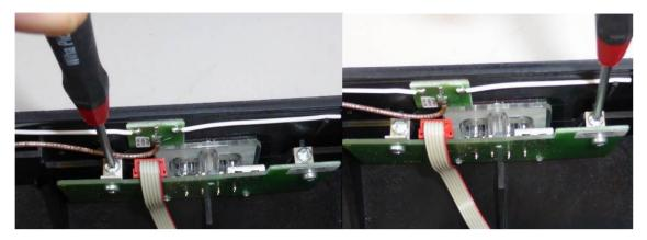
The module has to be connected electrically with the transmitter via BU1. So the connection cable has to be plugged in BU1.
