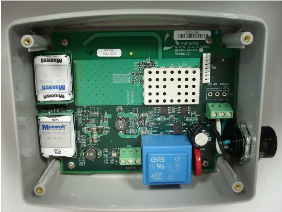
View of RepNode circuit board mounted inside enclosure
