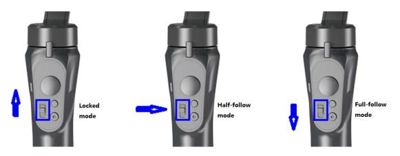
①Locked mode (the viewfinder screen does not follow the direction of rotation of the handle, and maintains a fixed direction): Mode switching switch slides to the top position, which is the locked mode.
