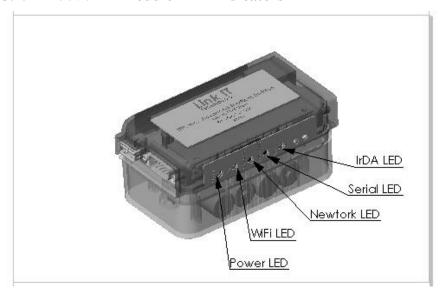
LEDs on the  $Link-iT^{TM}$  module indicate function or activity for specific aspects of the system.
