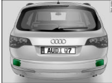
Fig. 178 Rear bumper: Position of radar sensors (not externally visible)
