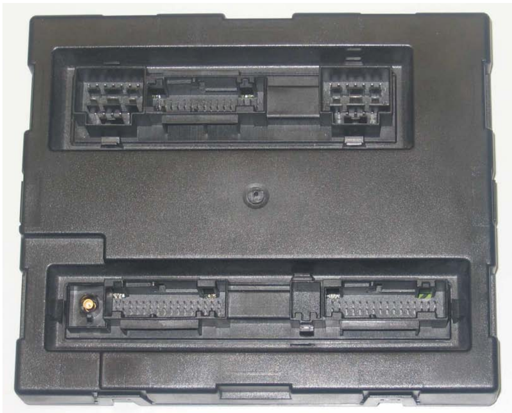
Picture 1: BCM2 with RF-connector down to the left
