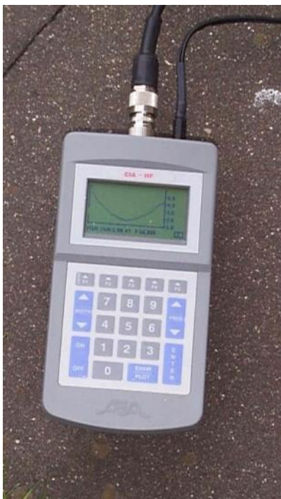
Antenna meter with broad resonance
