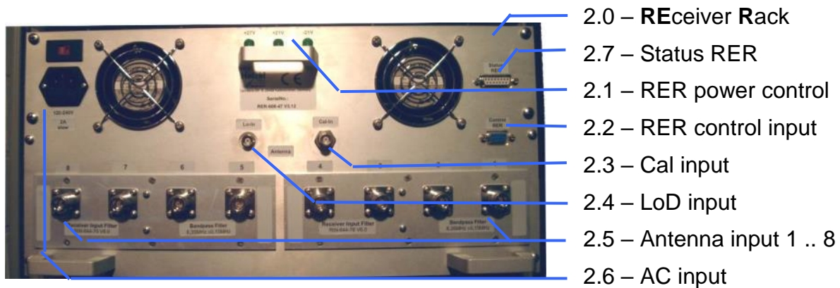
Figure 3.1: Back view, WERA RER internal Filters (8 channels)
