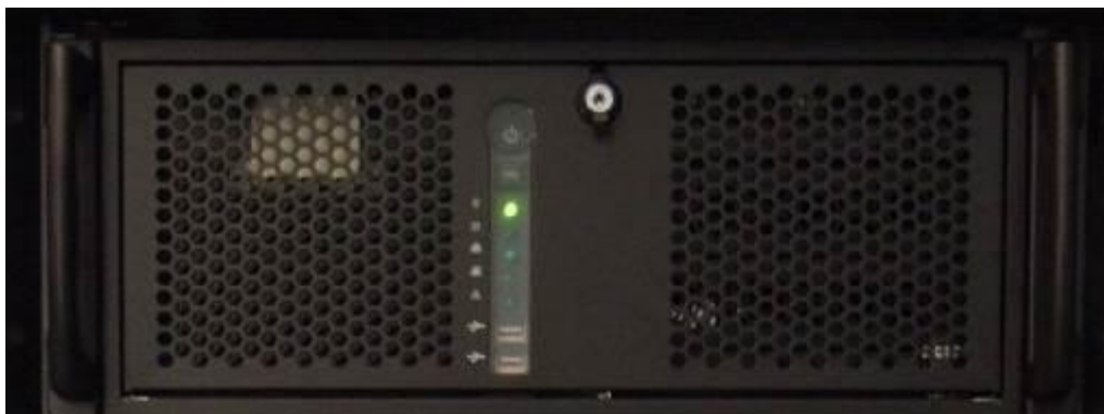
Figure 23: Typical User Interface PC (in this case with 3 height units, newer ones with 2 HU)
