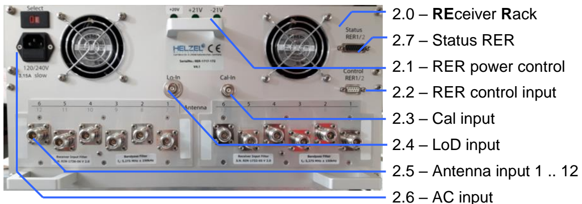
Figure 3.2: Back view, WERA RER (12 channels) – Version with internal Filters (RIN6)
