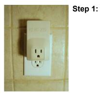
Plug the HEMS 220™ into the AC Wall Outlet first.
