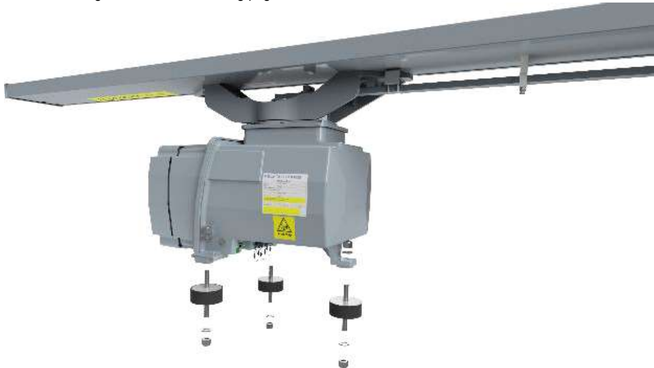
Mounting arrangement showing anti vibration mounts.
