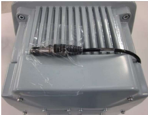
Example of fan power cable location
