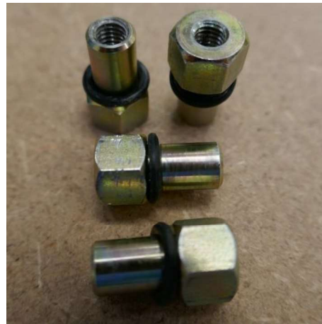
The four 10mm Sleeve nuts that retain the DC Motor
