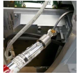
EXAMPLE of tightening an RF coupling to 0.9Nm
