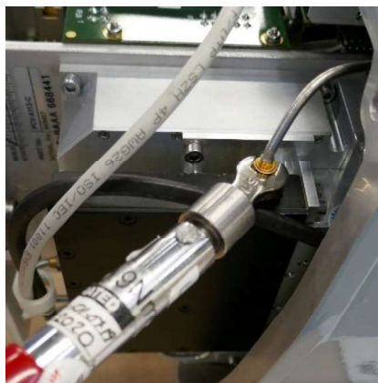
EXAMPLE of tightening an RF coupling to 0.9Nm
