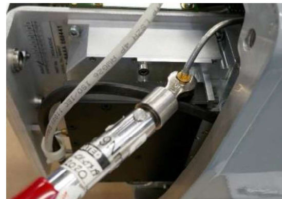
Tightening the RF coupling to 0.9Nm
