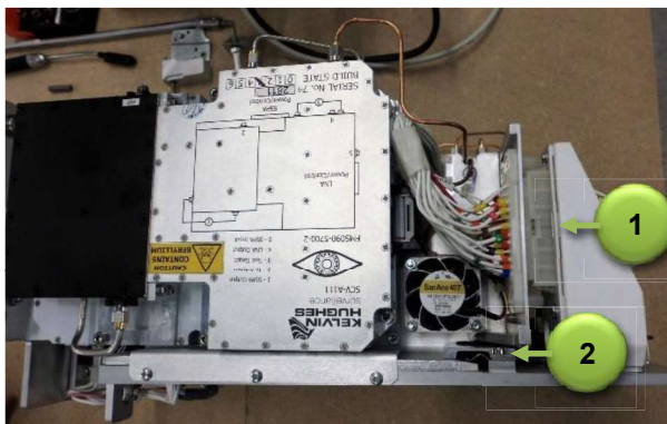
Example of the Transceiver Assembly mounted onto the Power Supply plate with the connectors (1) mated and the Transceiver Assembly located into the Power Supply restraining clamps (2).
