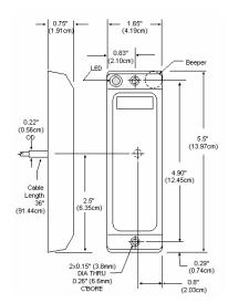
Route the cable through the center hole to the controller. Using the two 6-32 or M-3 screws attach the reader to the two mounting holes.
