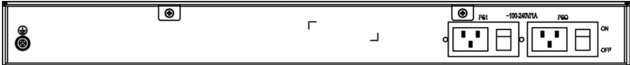
Figure 1-17: SG-6000-G2120/SG-6000-G2110 (dual power supply) Back Panel
