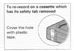
The VCR automatically enters the playback mode when a cassette without its safety tab is inserted. The VCR won't record on a tape without a safety tab and the cassette will be ejected if the REC or REC/IRT button is pressed. Be sure to check the safety tab before inserting a cassette.
