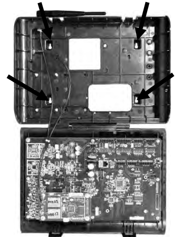
Figure 14. Open base station showing four screw holes
