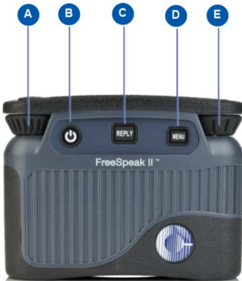
Figure 7-5 Beltpack front controls
