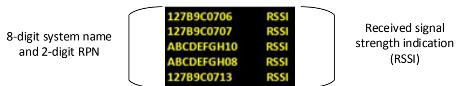
Figure 3-4 An unconnected beltpack site survey screen
