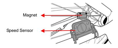
Note: There is a power button on the surface of the speed sensor. Do not push it unless you want to reset it.
