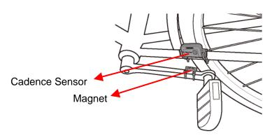
Note: There is a power button on the surface of the cadence sensor. Do not push it unless you want to reset it.
