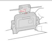
Thread and wind the included two cable ties (thicker ones) to secure the speed sensor onto the chain stay. Trim the cable ties if they hinder the rotation
