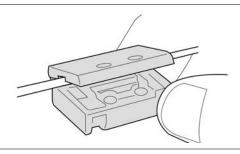
Place the speed sensor on the inner side of a chain stay. Make sure the speed sensor and the magnet should pass facing each other with no more than 25 millimeters between the two.
