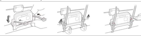
Secure the speed sensor to make sure it is firmly attached to the spoke without moving upward or downward while cycling.
