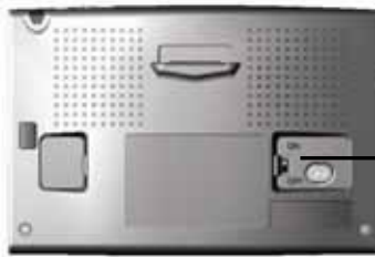
System Power switch
