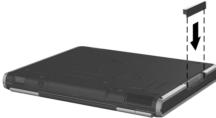
Replacing the hard drive bezel
