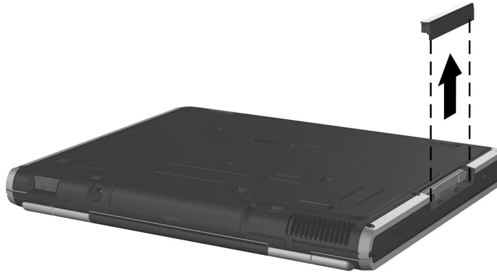
Removing the hard drive bezel
