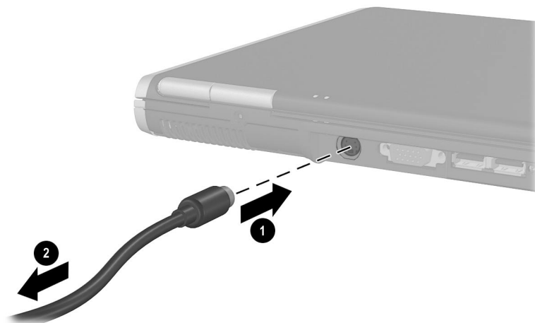
Connecting a device to the S-video-out jack
