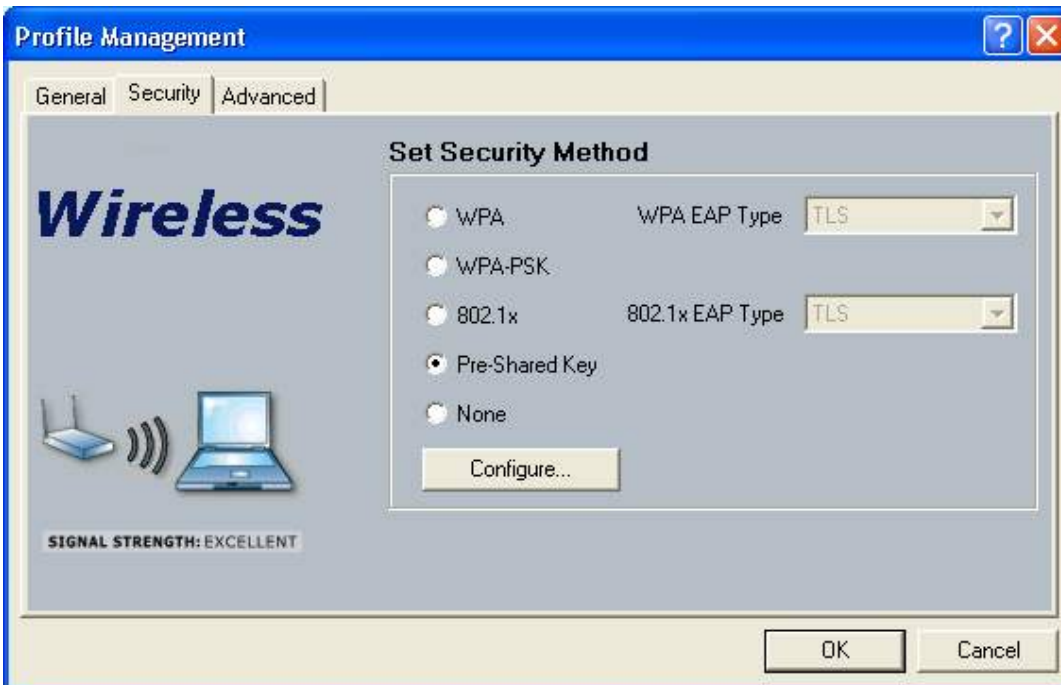
Figure 4-9 Security Setting under Profile Management Mode
