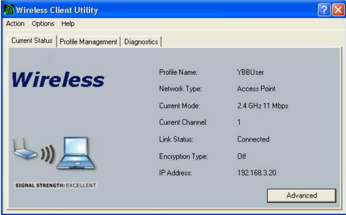
Figure 4-3 Current Status Tab Displays Current Wireless Connection
