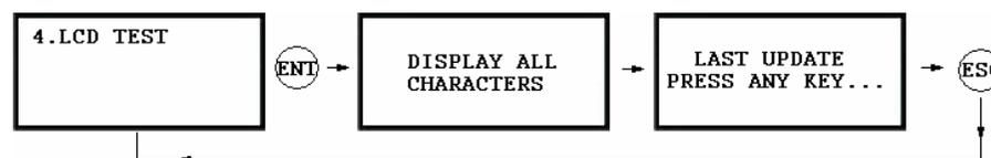
☞. The LCD will display all characters on the screen. When the test is done, the LCD will show "Last Update Press any key".
