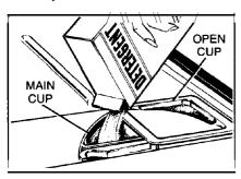
See c'Detergent Usage Guide" below. (Be sure the Cycle Indicator Dial is at **OFF position** before adding detergent. Otherwise the detergent cup will not close and latch properly.)
