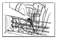
Remove the silverware basket and place a candy or meat thermometer in the water towards the middle of the tub. If the temperature is less than 120°F, you will not get good washing results. Higher water temperature is needed to dissolve grease and activate powder detergents.
