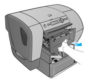
5 Look for the two guides inside the printer. Insert the rails of the auto-duplex unit into these guides. Slide the auto-duplex unit into the printer until it locks into place.
