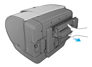
2 Slide the multipurpose tray into the Tray 1 opening at the back of the printer until it snaps into place.
