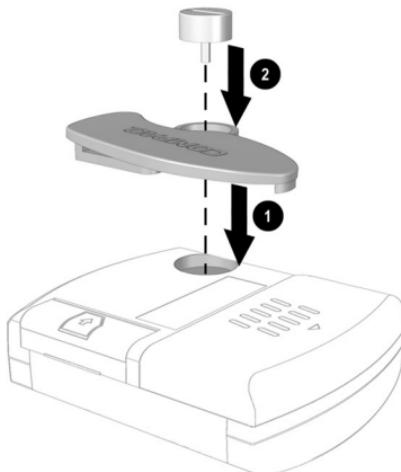
**Tip:** When installing new batteries, loosen the screw and rotate the belt clip clockwise, or remove the belt clip completely.
