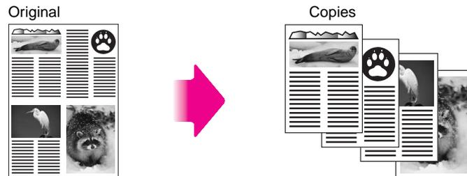
**Figure 37** Single-sided original divided into four equal sections
