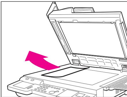
**6** Remove the originals from the glass and lower the optional ADF.
