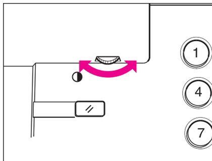
**Figure 9** Control panel display contrast adjustment
