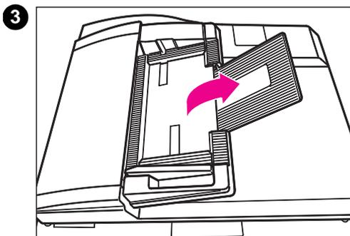
When you place several sheets of originals in the optional ADF and press **START**, they are automatically fed to the glass for copying. Double-sided originals are automatically flipped inside the optional ADF to make copies of both sides.
