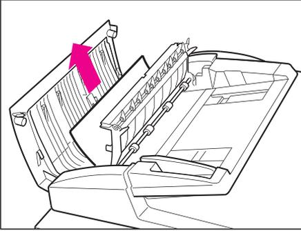
3 Open the inner cover, and remove the jammed originals. Close the inner cover after the jammed originals have been removed.
