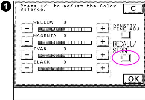
The copy module can store up to four color balance and color density settings you commonly use. You can access these settings through the copy module touch screen display.
