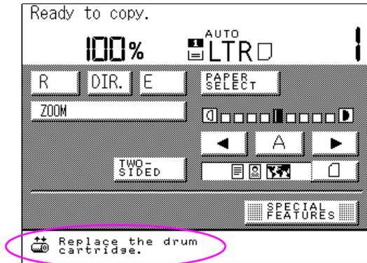
**Figure 59** Drum cartridge message - Basic Features screen
