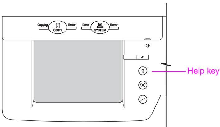
**Figure 8** Control panel Help key
