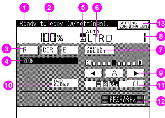
**Figure 10** Touch panel display—Basic Features screen
