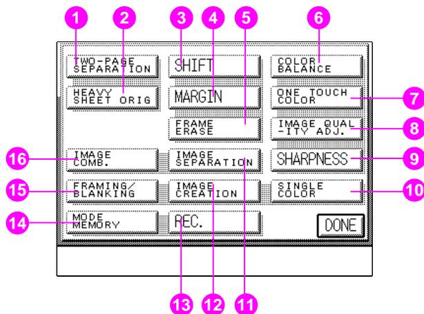
**Figure 11** Touch panel display—Special Features screen
