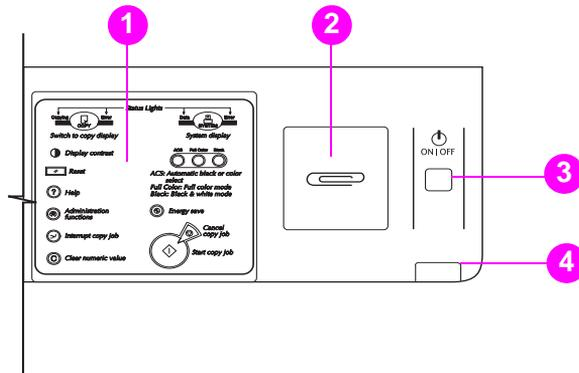
**Figure 4** Right-side view of copy module control panel
