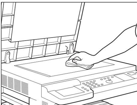
**Figure 64** Cleaning the copy module glass
