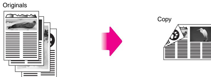
**Figure 35** Four originals copied onto the front and back of one sheet (2 on 1/two-sided mode)
