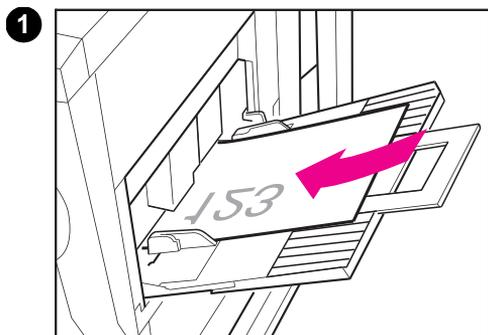
You can use Tray 1 to copy onto the second side of a sheet. However, the first side of the originals must have already been copied. Place originals with the printed side down in Tray 1.
