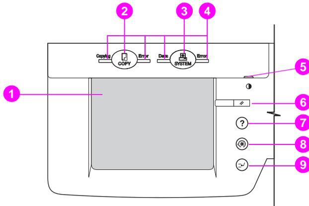
**Figure 5** Left-side view of the copy module control panel
