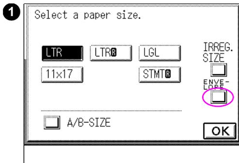
1 Load envelopes into Tray 1. (For more information on how to load envelope into Tray 1 see page 62.) In the paper size selection screen, press ENVELOPE. The envelope size selection screen appears.
