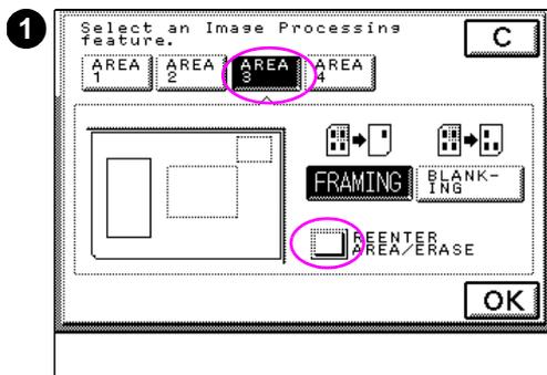
1 After you press FRAMING, select the button of the area to be cleared. Then press REENTER AREA/ERASE.
