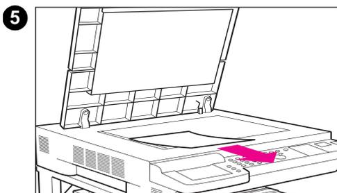
**5** When the Interrupt mode is canceled, lift the cover to remove the original copied in the Interrupt mode.
