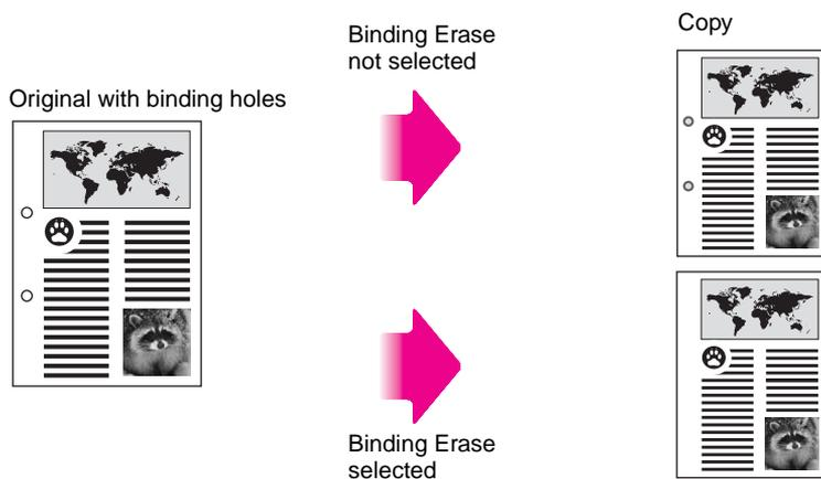
**Figure 33** Image without and with binding holes erased
