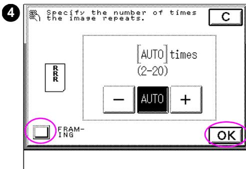
4 Specify the number of times you want the image to be repeated using the numeric keys or the - and + buttons. Press **AUTO** to make copies with the Auto Repeat setting. If you want to copy only a designated area of the original, press **FRAMING**. (See the framing instructions on page 165.) After completing the framing selection, or if you are not using framing, press **OK** and proceed to step 5.
