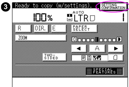
**3** To confirm the mode settings that cannot be confirmed in the Basic Features screen, press **SETTING CONFIRMATION**.
