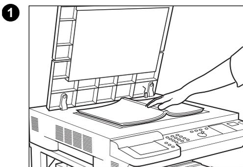
1 Place the original face down with the top edge resting against the back of the glass, away from the control panel.
