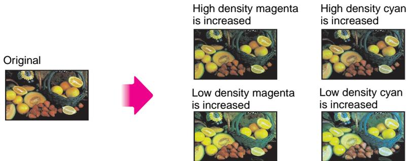
**Figure 49** Examples of Color Density adjustments
