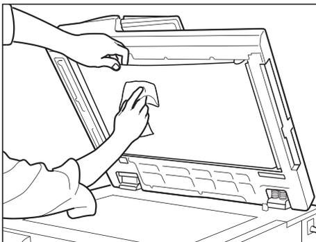
**Figure 66**      **Cleaning the feeding belt**
