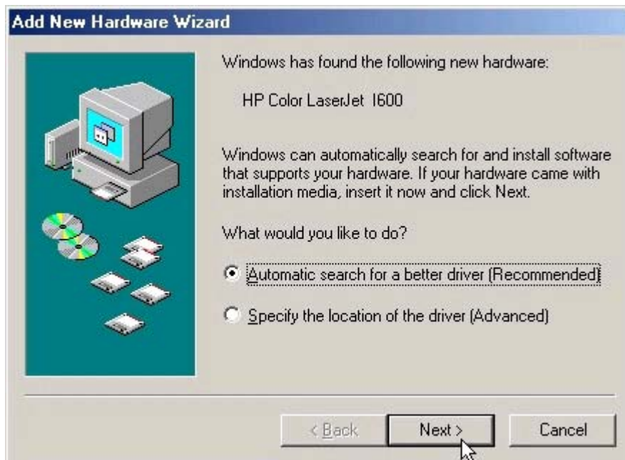
Figure 3-12 Add New Hardware Wizard USB Printing Support - Search for driver dialog box
